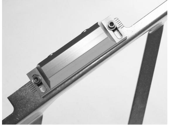
With referring to the scale, tilt the magnet plate. When the position is decided, fix the screws firmly.
