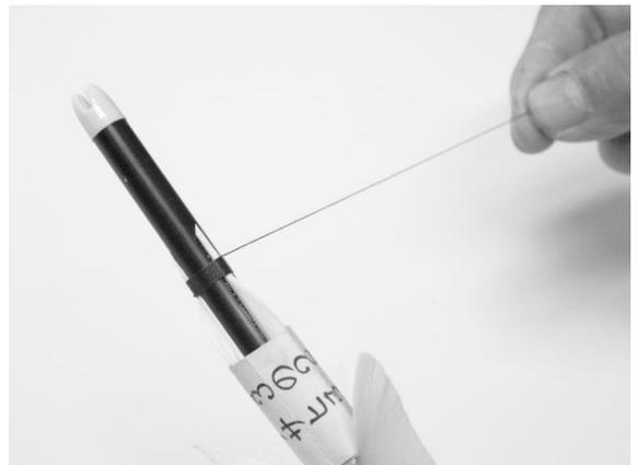
Wind the main thread toward the line drawn on figure #7. Leave no spaces.
