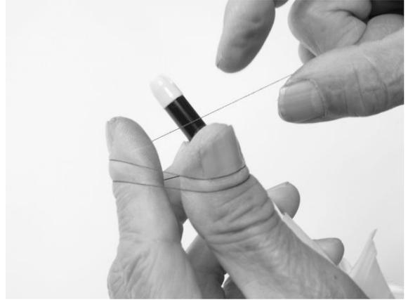
Hold the thread on the shaft with your middle finger and make a loop by winding the thread twice around your index finger and thumb.
