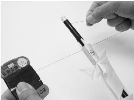
Cross the thread spool under the shaft and make a big loop while stretching the thread.
