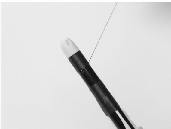
Hold the thread so it does not uncoil and pull it until it meets the line. Cut the leftover thread.
