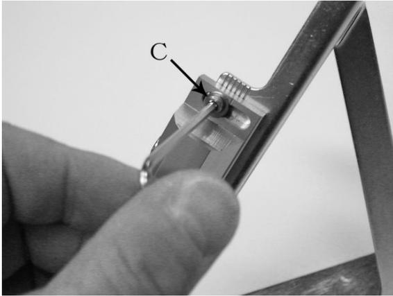
Unscrew the upper and lower screws (C) with the wrench provided in the box.
