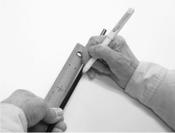
Measure the length of the arrow from the root of the nock and mark 1cm shorter than the desired arrow length.
