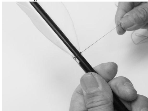
Begin to wind the thread at the feather line and keep winding without leaving spaces until it meets the line drawn in figure #7. When the thread reaches the line, wind 2 to 3 times.
