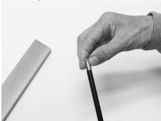
Partially insert a point on the shaft (it must be straight).
