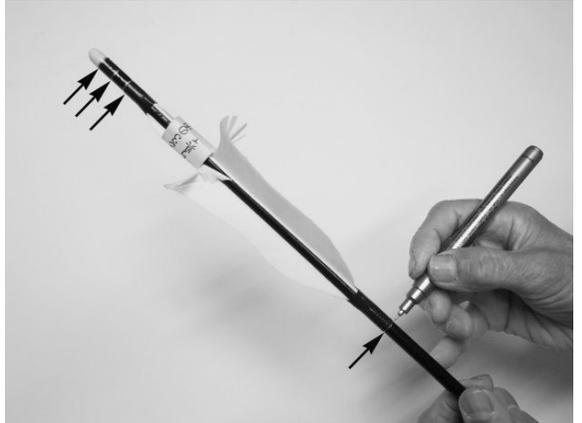
After the Urethane dries, draw finishing lines with a marker pen on the edges of the thread (shown by arrows).
